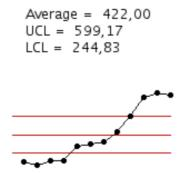
**Conclusion**. In this example, the control chart drawn according to the Shewhart method shows us that the process is not under control. On the contrary, the control limits calculated by using the « pocket calculator sigma » could make us think that it is under control.
